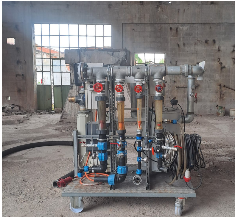
Figura 2: Impianto Soil Vapor Extraction (SVE)
